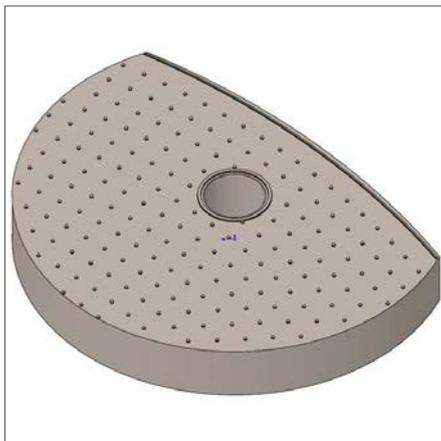
Fig.1: Cutout of a vacuum chuck surface, showing pins arranged concentrically around the center of the chuck, a hole with surrounding vacuum seal and a part of the edge vacuum seal.
